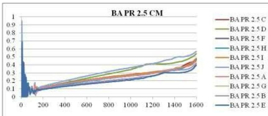
**FIGURE 9,** Curve Absorption Coefficient of 2.5 Cm Sample Thickness
