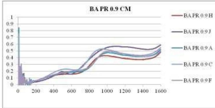
**FIGURE 4.** Curve Absorption Coefficient of 0.9 Cm Sample Thickness (Sample A-C-F-H-J)
