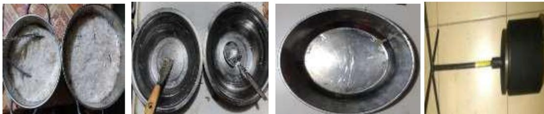
FIGURE 1. Aluminum pans and basins as a mixing medium for sample making work
