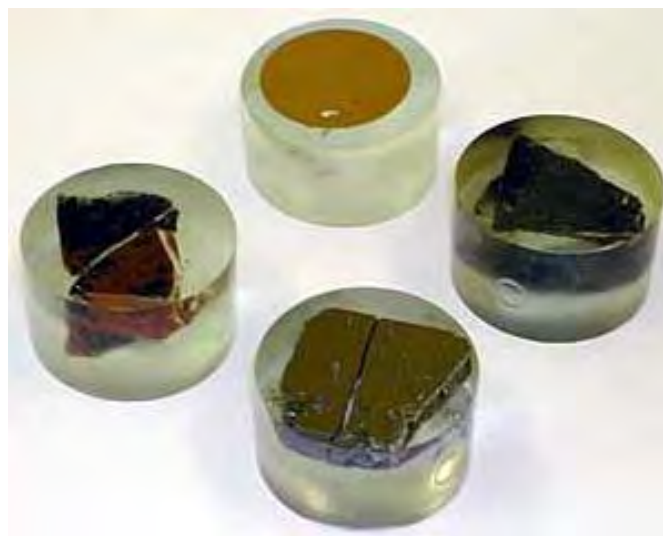
Gambar 3. Embedded/Mounted sampel batuan dan mineral (1-inc epoxy)
