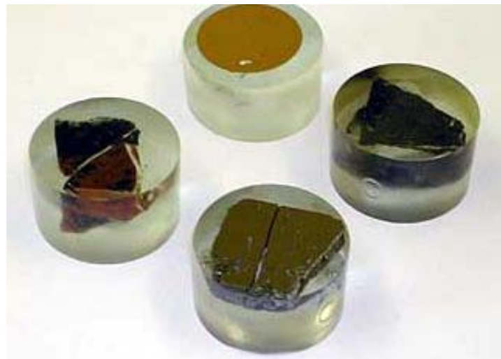
Gambar 3. Embedded/Mounted sampel batuan dan mineral (1-inc epoxy)
